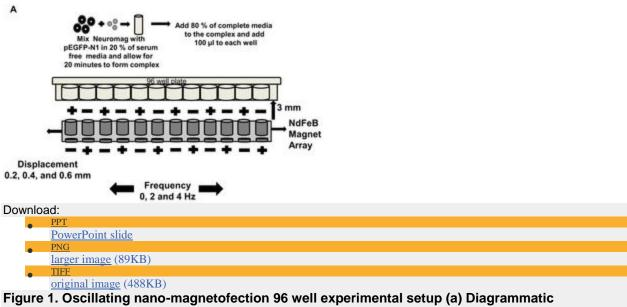
representation of a 96 well oscillating magnet array-based nanomagnetic transfection setup using NdFeB magnetic array.
